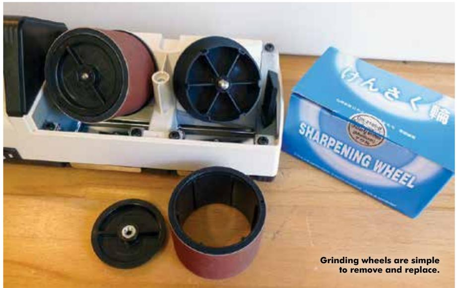
Grinding wheels are simple to remove and replace.
